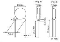
Lead Code Coating Extension e 0.6±0.05 Fig. 1 A2, A3 Up to the end of crimp C1, CD 3.0 max 0.5±0.05 Fig. 2 3.0 max 0.6±0.05 Fig. 2 C3
